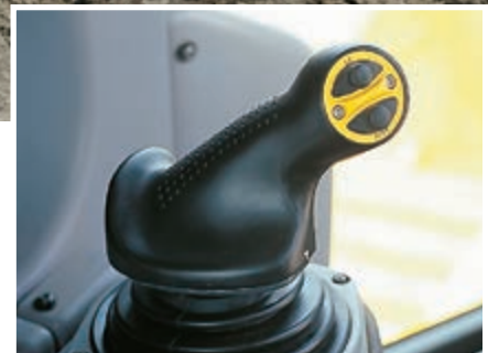
PCCS (Palm Command Control System)
